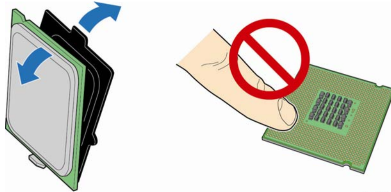
Figure 11. Remove the Processor from the Protective Processor Cover
